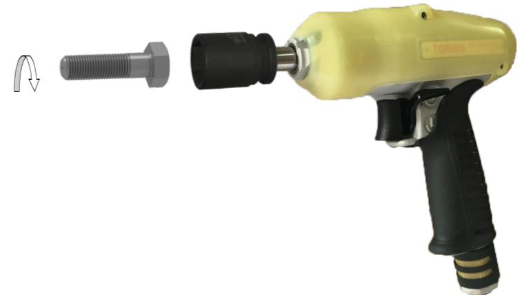
Reverse torque oil-pulse tool is available for reverse bolt.
