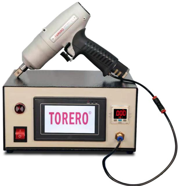
Pistol shut-off oil-pulse tool with a signal tube
