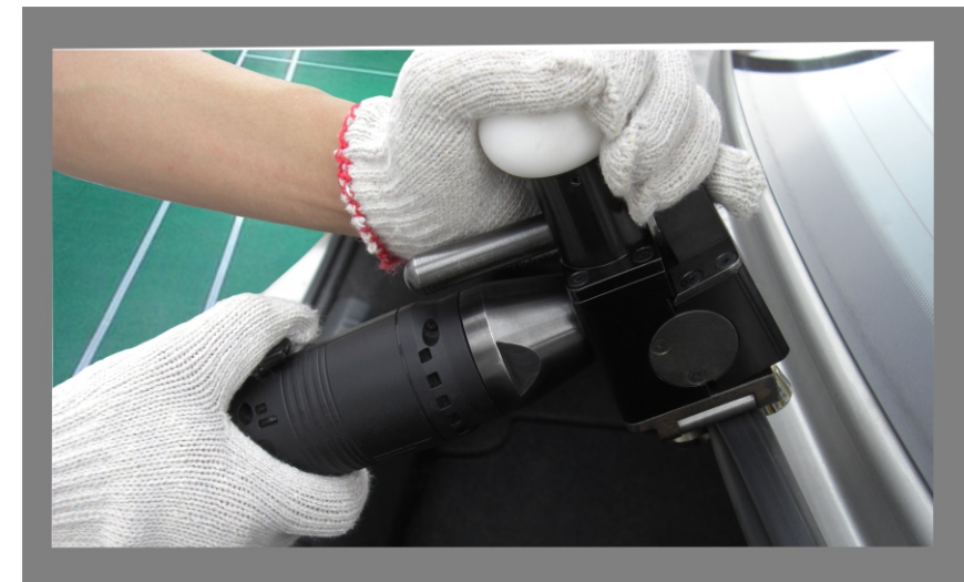
Model: ATV - 100SR Automobile Seal Strip Rolling Device
